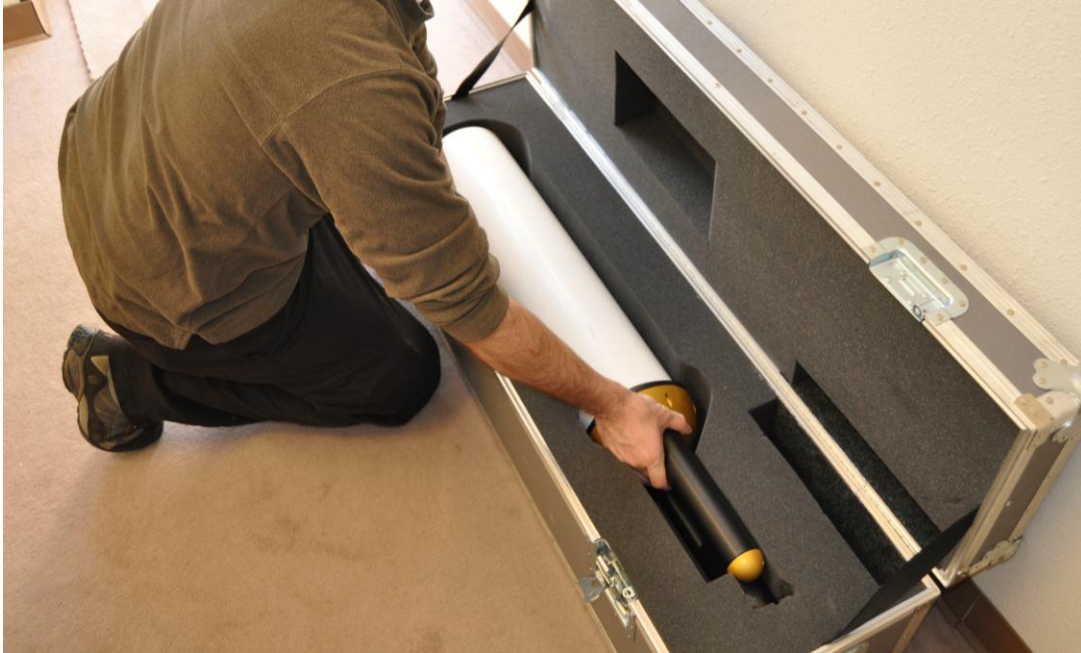
Figure 1.2 The FFSSP being removed from the shipping case, held by the arm and main body. The arm should only be held in the position shown and never close to the tips. The main body should not be held by the connector.
