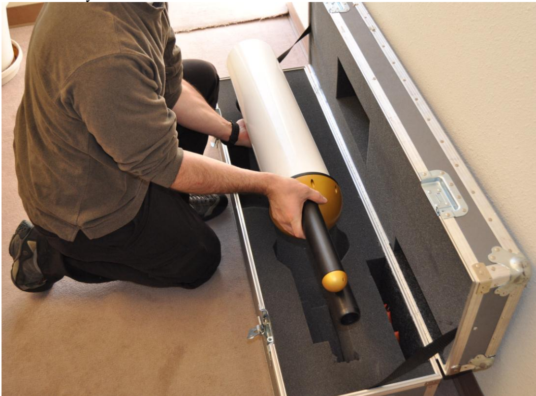
Figure 1.2 The FFSSP being removed from the shipping case, held by the arm and main body. The arm should only be held in the position shown and never close to the tips. The main body should not be held by the connector.
