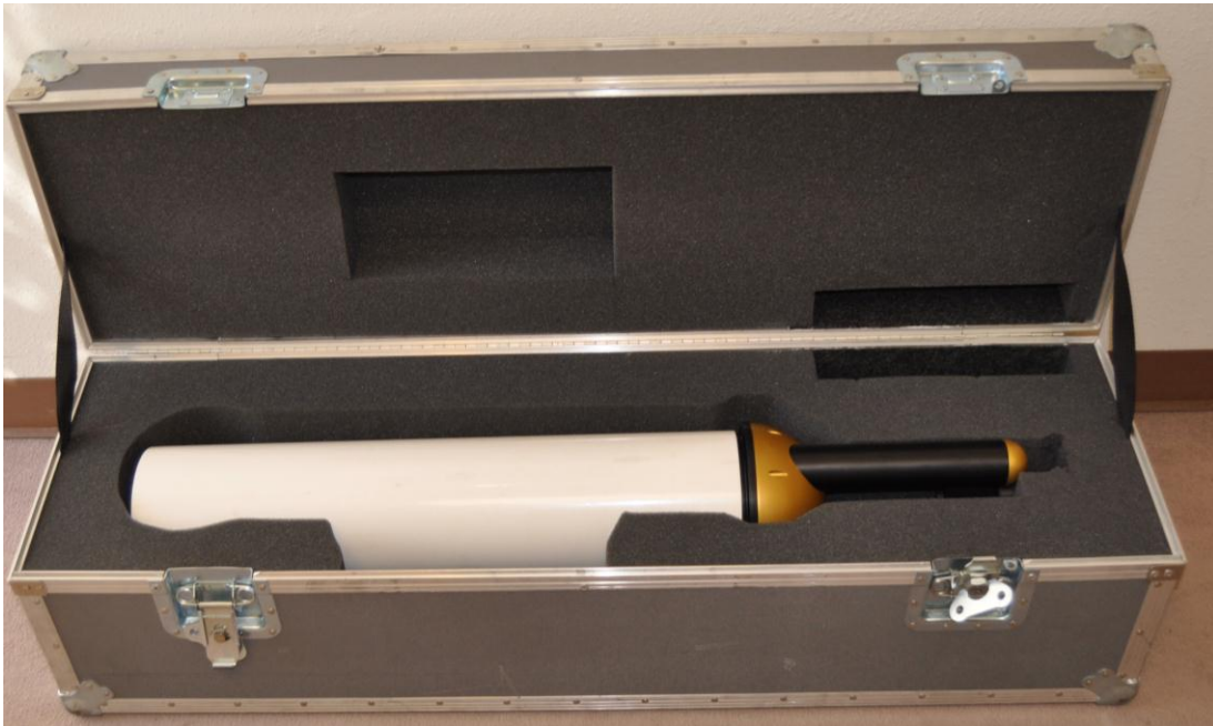
Figure 1.1 The FFSSP in a shock-absorbing foam protected shipping case
